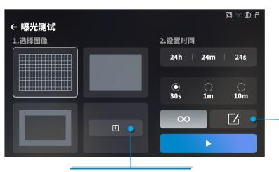
Custom exposure time : Can be exposed all the time, for screen aging and other tests.
